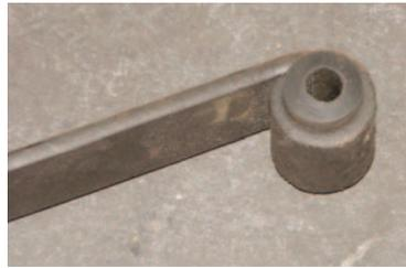
**Photo #10:** This is a good time to check your rear shackle bushings. The 1955 shackle uses the P/N 21-235 bushing set. The 1956 and 57 shackle uses the P/N 21-236 bushing set.
