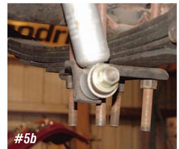
**Photo #5a & 5b:** The rear end housing is held to the leaf springs with two U-bolts on each side. The U-bolts wrap around the rear end and hold the lower shock plate in place.
