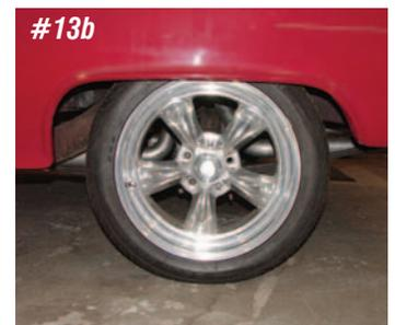
**Photo #13a & 13b:** Install the wheels and tires and sit the car on the ground. Bounce the car several times allowing the leaf spring bushings to seat into place. Now tighten the front leaf spring mounting bolts and the rear shackle nuts. The front mounting bolts torque to 60-90 ft/lbs, while the rear shackle nuts torque to 25-30 ft/lbs.
