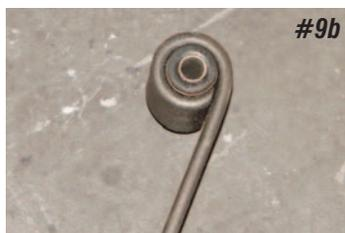
**Photo #9a & 9b:** We are installing the 5-leaf, 2" lowering spring P/N 21-262. The rear spring eye is inverted to lower a passenger car 2". The new spring includes the forward eye bushing.
