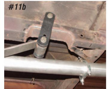
**Photo #11a & 11b:** Install the new leaf springs, leaving the front nut and bolt and shackle nuts loose at this time.
