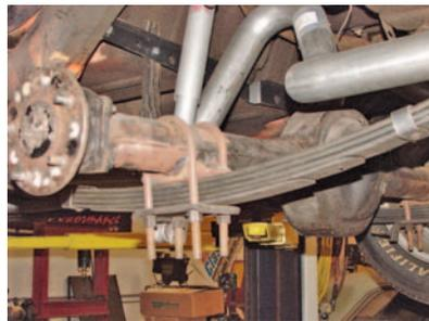
**Photo #12:** Lower the rear end down onto the spring center bolt and install the U-bolts, lower shock plates and shock absorbers. Torque the U-bolt nuts to 45-55 ft/lbs and torque the shock absorber nut to 35 ft/lbs.
