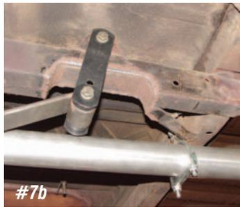
**Photo #7a & 7b:** The leaf spring is anchored to a bracket on the frame in the front with a single 1/2" bolt and to the rear of the frame with a shackle. Our project car has the CCI Spring Pocket Kit P/N 21-131 that mounts the leaf spring parallel with the frame rails allowing for a larger tire. The removable of the leaf springs will be the same procedure as stock.
