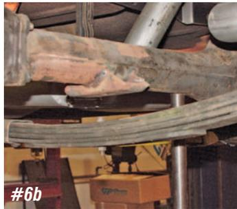
**Photo #6a & 6b:** With the frame on jack stands or the car raised on a lift, remove the shock absorber. Next remove the four nuts from the U-bolts and raise the rear end off the leaf spring one side of the car at a time.
