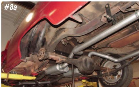
**Photo #8a & 8b:** Remove the front bolt and the rear shackle so the leaf spring can be removed from the frame.
