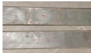
**Photo #4:** The offset leaf spring has the spring center pin moved to the rear of the spring 3/4" compared to the stock spring.
