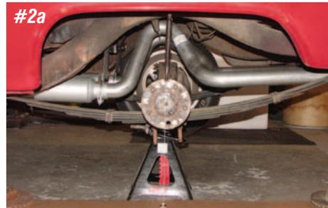
**Photo #2a & 2b:** On our 1955 we dropped a plum bob off the front and rear wheel openings and off the center line of the rear end. With the rear in the stock location, you will find that it is 1" closer to the front of the wheel opening than the rear.
