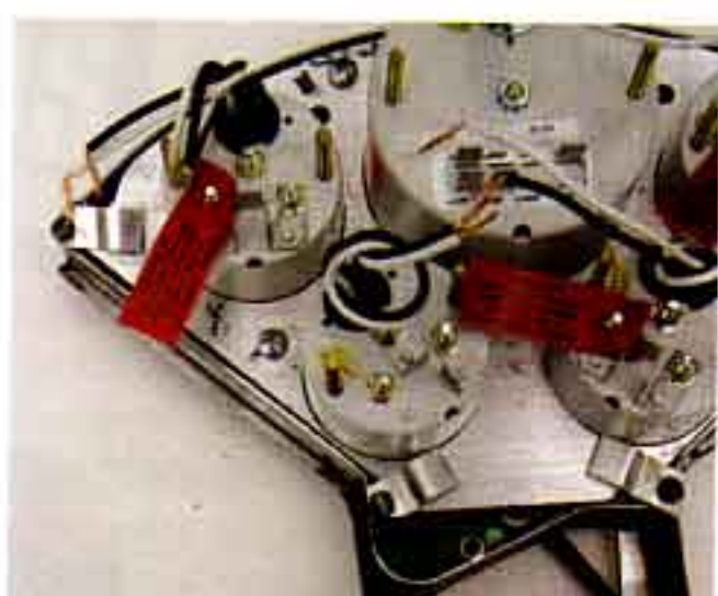
Photo #4a & 4b: The gauge cluster is held into the original chrome instrument bezel with five tabs supplied with the kit. Using the original five machine screws, anchor the panel into place. The edge of the tabs will need to be trimmed so the instrument bezel assembly will slide back into the dash board.
