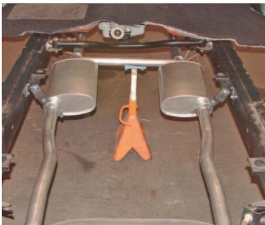
**Photo #13:** The tailpipes slip into the muffler outlets and are held to the mufflers using the same clamps on the muffler hangers.
