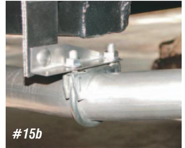
**Photo #15a & 15b:** The tailpipe hanger has a rubber strap with a steel tab to fit under the muffler clamp. Mount the hanger to the rear of the bracket and using the supplied muffler clamp, bolt the tailpipe in place. The tailpipes on the performance systems run between the rear end and the shocks while stock systems run between the shocks and the frame.
