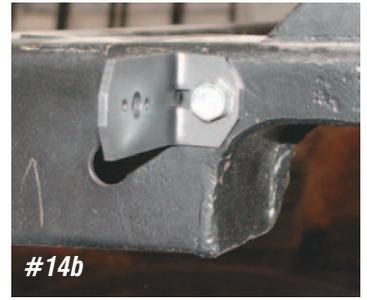
**Photo #14a & 14b:** The tailpipe hangers are held to the frame using stock dual exhaust tailpipe hanger brackets, also included in the new exhaust system. The brackets are bolted to the frame just behind the rear shackle mounts using one bolt into the frame. There are two holes in the frame; one for the mounting bolt and one for the locating tab on the bracket.
