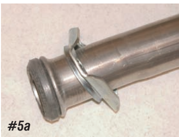
Photo #5a & 5b: The exhaust donut fits on the collar of the exhaust pipe and seats on the ring of the pipe for a leak-proof seal. The exhaust pipe flange includes a collar. When properly installed, the collar fits the ring on the exhaust pipe. Install the driver's side exhaust pipe to the manifold leaving the three nuts loose at this time.
