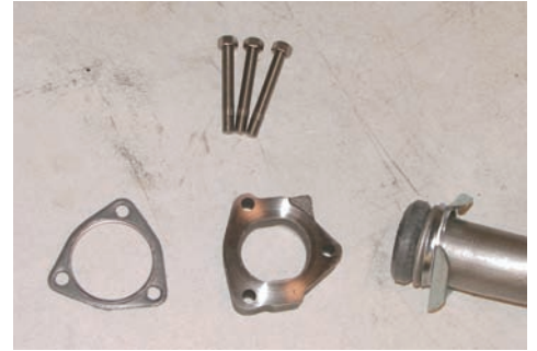
Photo #6: The passenger side exhaust manifold always uses a heat riser. A heat riser P/N 24-01 or heat riser delete P/N 24-03 must be used to properly space the exhaust pipe so it will line up with the rest of the exhaust system.
