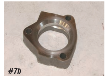
Photo #7a & 7b: The heat riser or heat riser delete is flat on one side and concave on the other. The flat side fits the exhaust manifold and the concave side fits the exhaust pipe donut.
