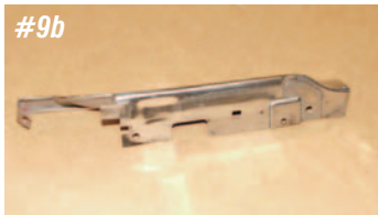
Photo #9a & 9b: The last piece of beltline stainless to install is the outer lower vent window stainless. The stainless molding is held to the door with three #6 countersunk sheet metal screws; two behind the vent window frame and one in the door jam.
