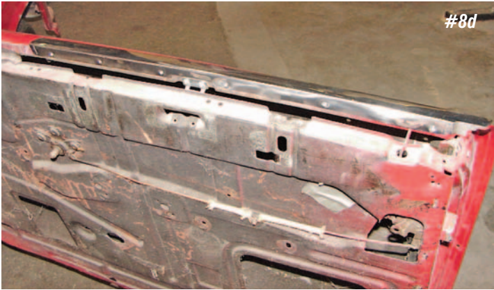
Photo #8a & 8b & 8c & 8d: The door window beltline moldings are held to the door with six #6 countersunk sheet metal screws included in kit P/N 34-38 . These outer door moldings do not receive whisker strips.
