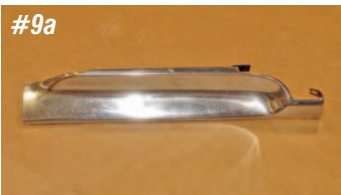
Photo #9a & 9b: The last piece of beltline stainless to install is the outer lower vent window stainless. The stainless molding is held to the door with three #6 countersunk sheet metal screws; two behind the vent window frame and one in the door jam.
