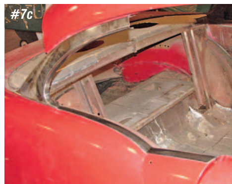
Photo #7a & 7b & 7c: The slots in the original beltline moldings are sometimes damaged. A new hole can be drilled in the molding and body to hold the moldings in place if needed.
