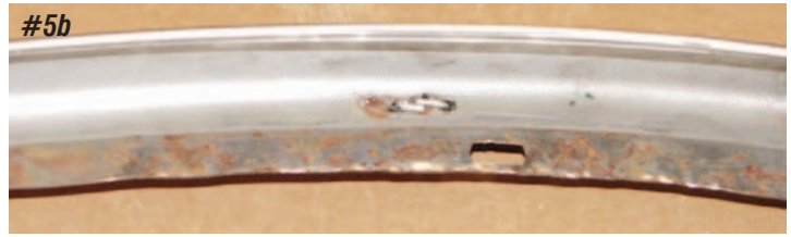
Photo #5a & 5b: The quarter window beltline moldings have a whisker strip stapled to the inner edge of the molding.
