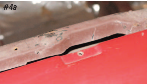
Photo #4a & 4b & 4c & 4d: At the front of the dogleg, there is a single hole. There is an impression in the top of the quarter panel that will match the hole in the dogleg. A #6 countersunk sheet metal screw, included in kit P/N 34-301 is used to hold the front of the molding in place. The rear tab on the
