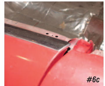
Photo #6a & 6b & 6c: The quarter window beltline moldings are held to the body with six #6 button head sheet metal screws kit P/N 34-113 . There are slots in the molding for front to rear adjustment.
