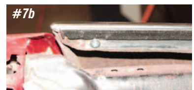
Photo #7a & 7b & 7c: The slots in the original beltline moldings are sometimes damaged. A new hole can be drilled in the molding and body to hold the moldings in place if needed.
