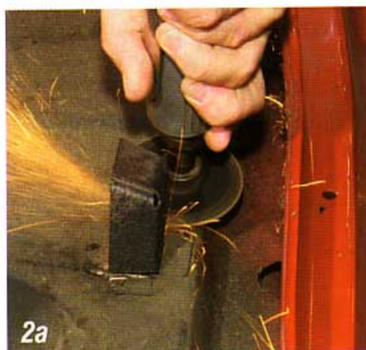
Photo #2a & 2b: The rear mounting pocket for the bumper jack and the tab for the spare tire hold down bolt will need to be removed to allow the trunk floor panel to lay flat.
