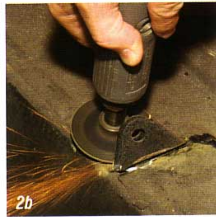
Photo #2a & 2b: The rear mounting pocket for the bumper jack and the tab for the spare tire hold down bolt will need to be removed to allow the trunk floor panel to lay flat.
