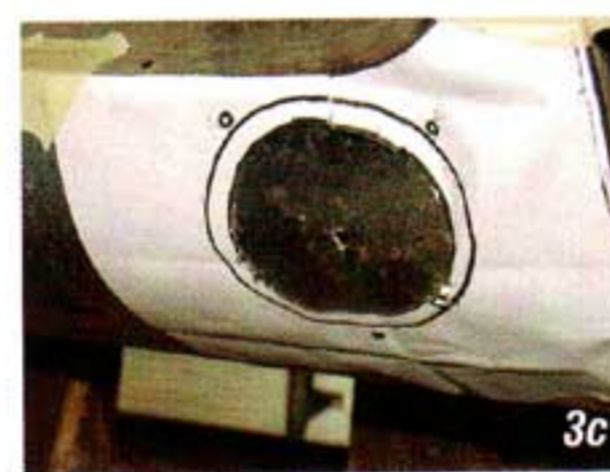
Photo #3a, 3b, 3c & 3d: A 3-1/2" metal hole saw is used to cut through the dash. At a low drill speed and light pressure, drill through the dash.
