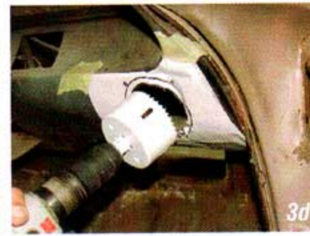
Photo #3a, 3b, 3c & 3d: A 3-1/2" metal hole saw is used to cut through the dash. At a low drill speed and light pressure, drill through the dash.
