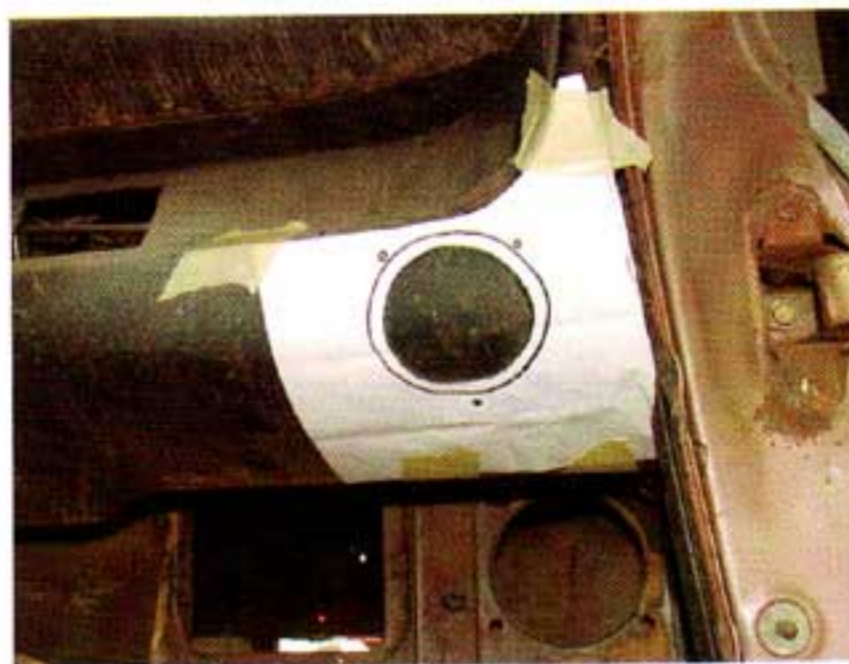
Photo #2: The outer edges of the template line up with the bottom of the dash, the edge of the dash where the dash trim is installed and the outer edge of the dash. Use masking tape to hold the template in place.
