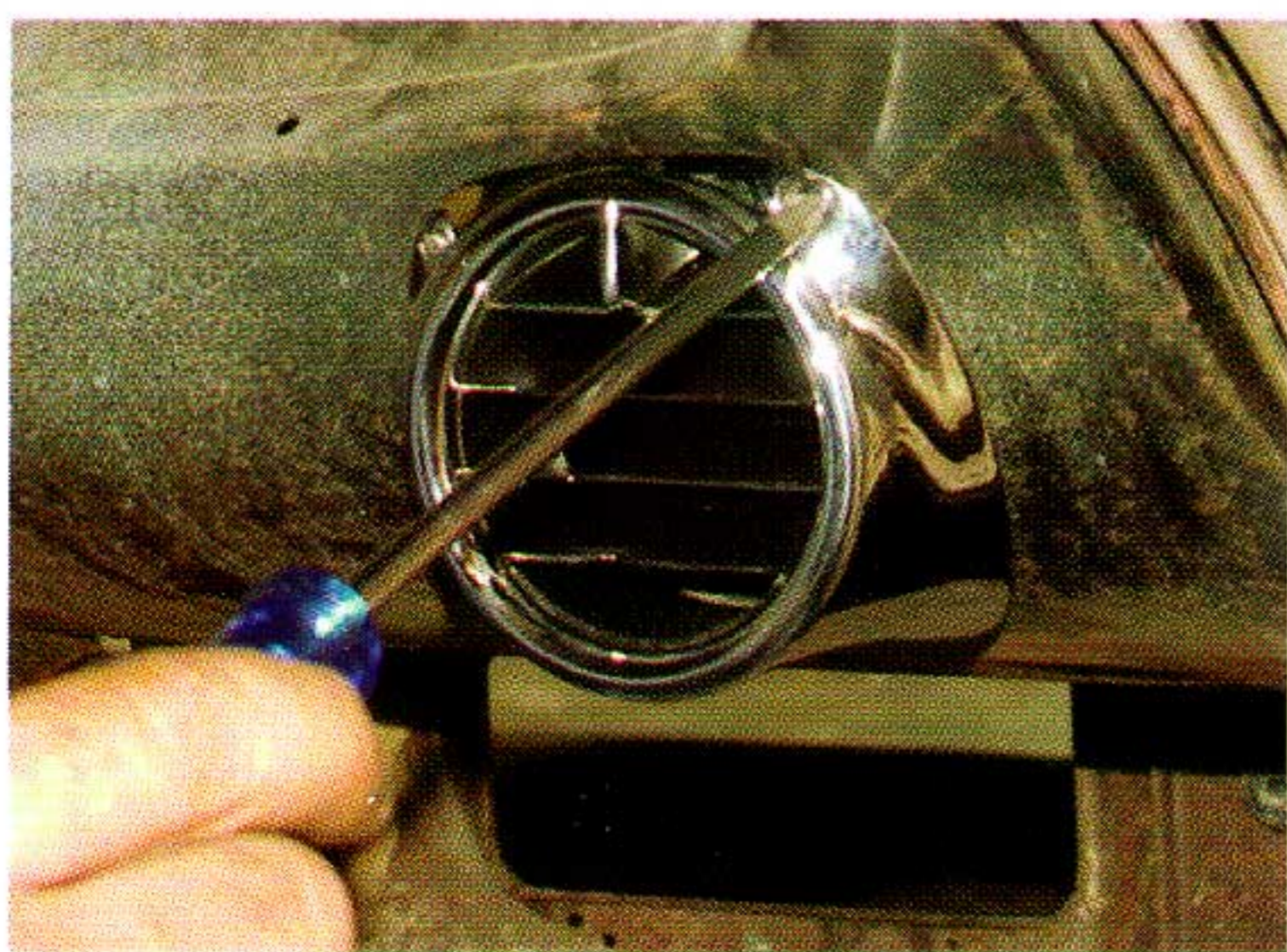
Photo #7: Next install the three #6 counter-sunk sheet metal screws and check the fit to the dash board. Repeat for the other side.
