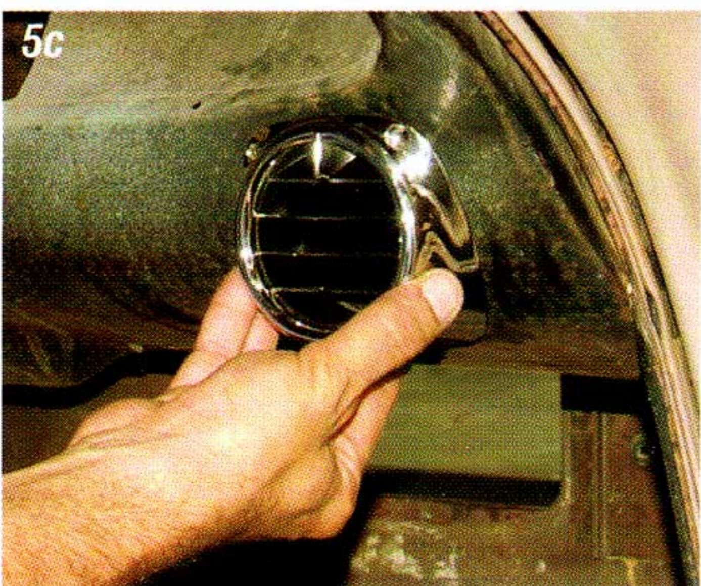
Photo #5a, 5b & 5c: Clean up the rough edges of the cut until you get a perfect fit.
