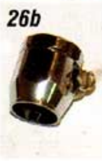
Photo #26a, 26b & 26c: The return hose from the steering box connects to the nipple on the back of the power steering pump reservoir. The hose kit includes a shielded hose clamp for this end. Cut the return hose to length using the electrical tape/chisel method and connect to the reservoir.
