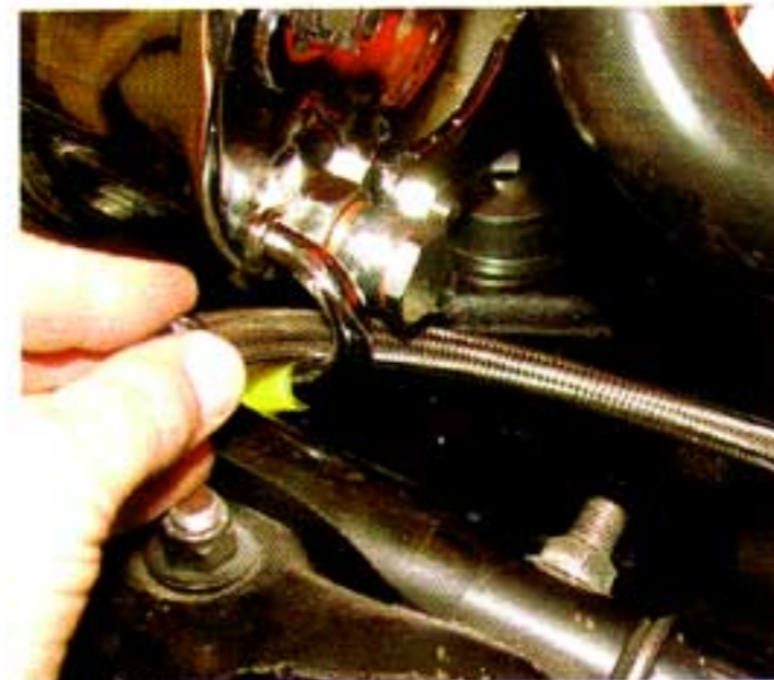
Photo #19: The banjo fitting screws into the pressure line port in the back of the power steering pump. Orient the fitting so that the line will clear any moving suspension parts or any hot exhaust parts. With the fitting installed in the steering box, hold the steel braided hose next to the banjo fitting on the power steering pump and mark the hose where it will need to be cut. The hose is made extra long so that it will work with a small block or big block engine.
