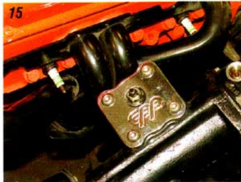
Photo #14 & 15b: A cover for the 670 power steering box is available in polished aluminum P/N 53-311 or brushed aluminum P/N 53-312 and includes four stainless button head bolts and lock washers.
