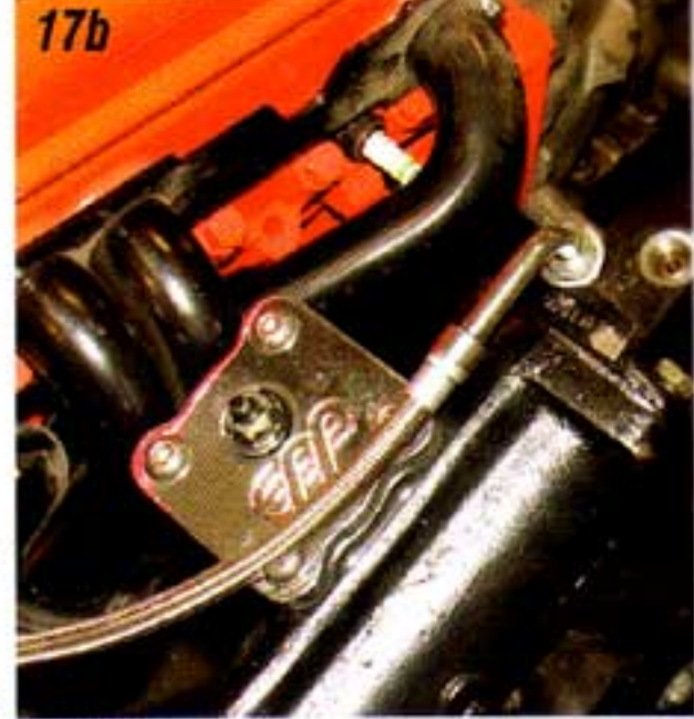
Photo #17a & 17b: The 605 and 670 power steering boxes have inverted flare fittings. The inner fitting closest to the engine is for the pressure hose.
