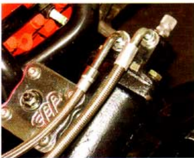
Photo #24a, 24b & 24c: Install the stem of the banjo fitting into the hose and tighten the locking nut onto the banjo fitting until the nut bottoms out. Now the banjo fitting can be installed back onto the power steering pump.
