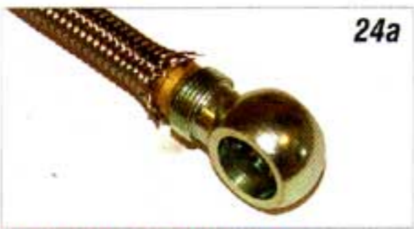
Photo #24a, 24b & 24c: Install the stem of the banjo fitting into the hose and tighten the locking nut onto the banjo fitting until the nut bottoms out. Now the banjo fitting can be installed back onto the power steering pump.
