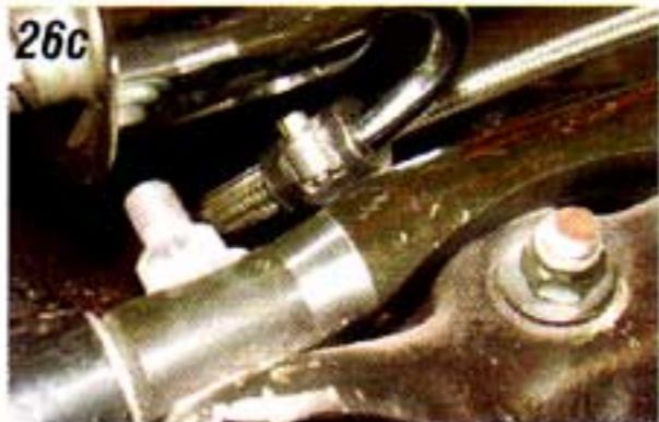
Photo #26a, 26b & 26c: The return hose from the steering box connects to the nipple on the back of the power steering pump reservoir. The hose kit includes a shielded hose clamp for this end. Cut the return hose to length using the electrical tape/chisel method and connect to the reservoir.
