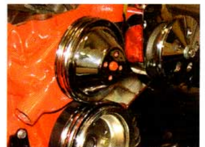
Photo #12: If air conditioning is installed, a double groove pulley P/N 211-19 must be used on the water pump. If air conditioning is not used a single groove pulley P/N 211-18 may be used.
