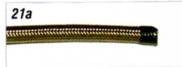
Photo #21a & 21b: After marking the steel braided hose, wrap it with electrical tape. This will keep the steel braid from fraying when the hose is cut. Before cutting the hose, install the locking nut for the banjo fitting. The steel braided hoses are Teflon, not rubber, so the hoses must be cut with a blade that will not create any heat. A sharp chisel works great!
