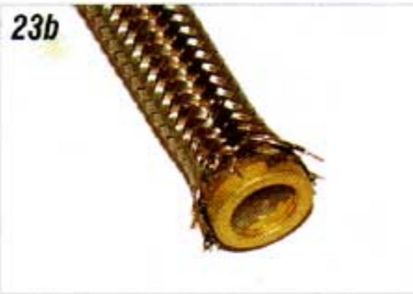
Photo #23a & 23b: Using a small flat blade screwdriver, separate the outer steel braid from the inner Teflon hose and install the ferrule for the banjo fitting over the hose.
