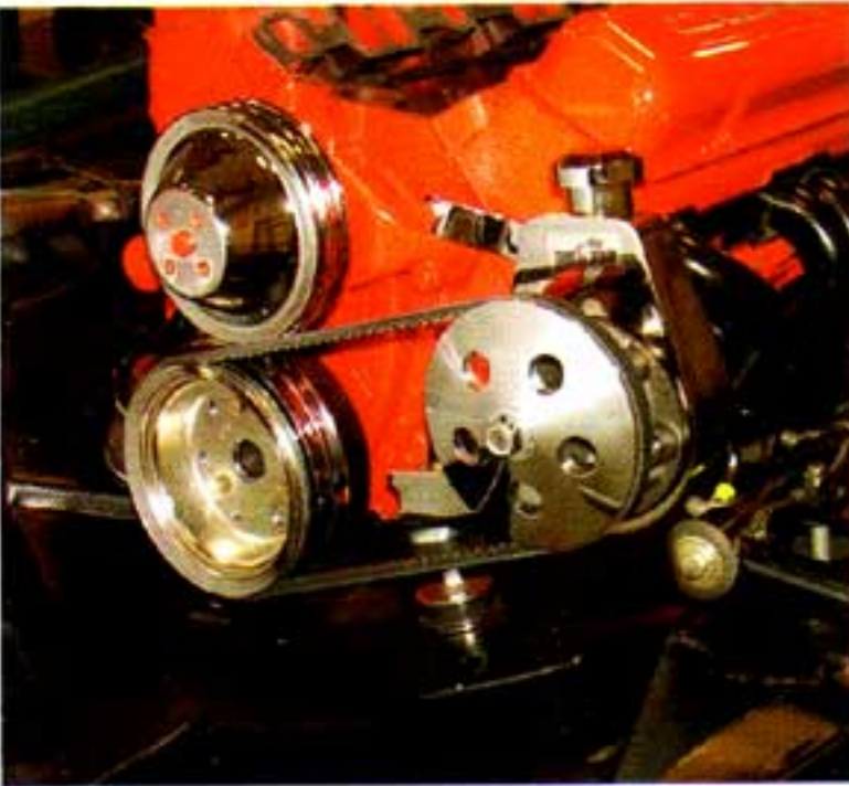
Photo #13: The fan belt P/N 41-12 may now be installed. With the power steering pump adjusted the pump will lean to the inside slightly. This will allow for clearance between the forward upper control arm stud and the pump reservoir.
