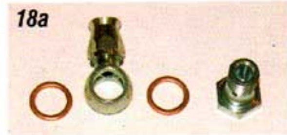
on the pressure hose. This will allow the hose to be oriented in any position to clear the exhaust or steering components. The hose kit includes a banjo bolt, two copper washers and a banjo block for the end of the hose.
