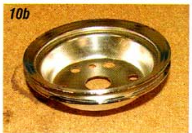
Photo #10a, 10b & 10c: The third groove on the crankshaft pulley (farthest out from the timing cover) is used to drive the power steering pump. The first groove is for the alternator and the second groove is for the air conditioning. A one-piece double-groove chrome pulley P/N 211-21 is used for the first and second groove. For the third groove a separate chrome pulley P/N 53-34C is used. The P/N 53-34C pulley fits inside the P/N 211-21 pulley to make up the three grooves.
