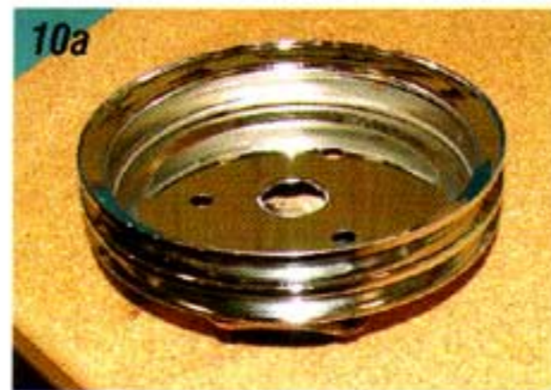
Photo #10a, 10b & 10c: The third groove on the crankshaft pulley (farthest out from the timing cover) is used to drive the power steering pump. The first groove is for the alternator and the second groove is for the air conditioning. A one-piece double-groove chrome pulley P/N 211-21 is used for the first and second groove. For the third groove a separate chrome pulley P/N 53-34C is used. The P/N 53-34C pulley fits inside the P/N 211-21 pulley to make up the three grooves.
