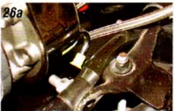
Photo #26a, 26b & 26c: The return hose from the steering box connects to the nipple on the back of the power steering pump reservoir. The hose kit includes a shielded hose clamp for this end. Cut the return hose to length using the electrical tape/chisel method and connect to the reservoir.
