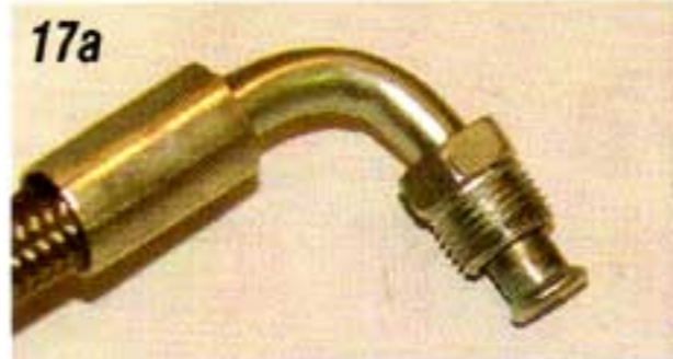
Photo #17a & 17b: The 605 and 670 power steering boxes have inverted flare fittings. The inner fitting closest to the engine is for the pressure hose.
