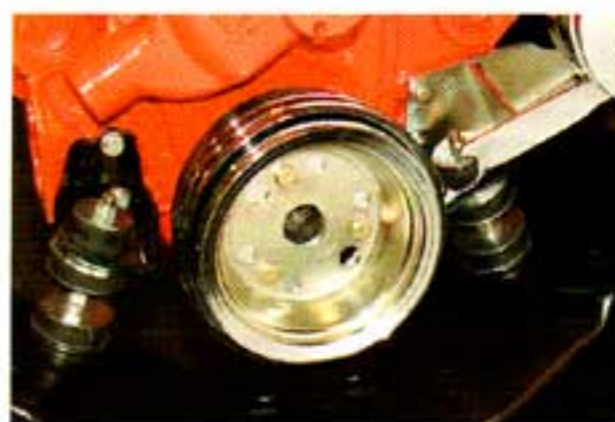
Photo #10a, 10b & 10c: The third groove on the crankshaft pulley (farthest out from the timing cover) is used to drive the power steering pump. The first groove is for the alternator and the second groove is for the air conditioning. A one-piece double-groove chrome pulley P/N 211-21 is used for the first and second groove. For the third groove a separate chrome pulley P/N 53-34C is used. The P/N 53-34C pulley fits inside the P/N 211-21 pulley to make up the three grooves.
