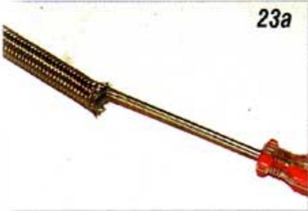
Photo #23a & 23b: Using a small flat blade screwdriver, separate the outer steel braid from the inner Teflon hose and install the ferrule for the banjo fitting over the hose.
