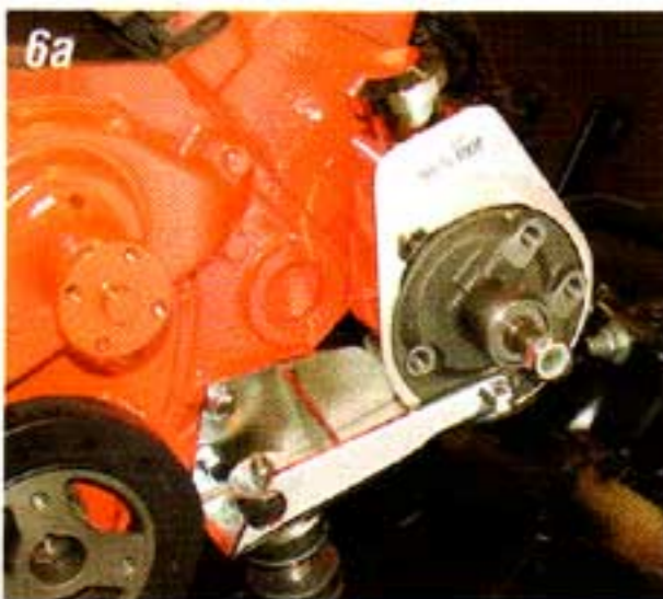
Photo #6a & 6b: The chrome power steering pump P/N 207-43 bolts to the new power steering bracket with a chrome 9/16" X 1" bolt, flat washer and lock washer. The rear of the pump has a stud that fits in a groove in the back of the bracket. The rear stud is secured to the bracket with a chrome nut, flat washer and lock washer.
