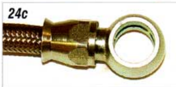
Photo #24a, 24b & 24c: Install the stem of the banjo fitting into the hose and tighten the locking nut onto the banjo fitting until the nut bottoms out. Now the banjo fitting can be installed back onto the power steering pump.
