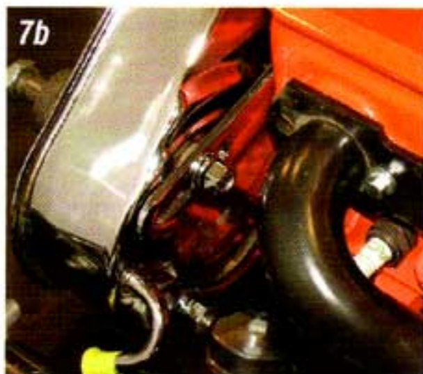
Photo #7a & 7b: The adjusting bracket P/N 53-29C for the power steering pump bolts to the upper water pump bolt on the driver's side of the engine. The adjusting slot fits onto the upper rear stud on the back of the power steering pump. A chrome 9/16" nut, flat washer and lock washer for the adjusting slot is included with the P/N 53-27C bracket kit.
