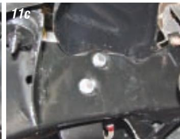
**Photos 11a, 11b & 11c:** If you measure ten different frames between the frame rails, you will get ten different measurements. The ears on the crossmember are leaned in at the top to accommodate for this variation. When the crossmember is bolted to the frame, the ears will pull into place and the frame will not move. The crossmember is held to the frame with 3/8" X 4" bolts with flat washers and lock nuts.
