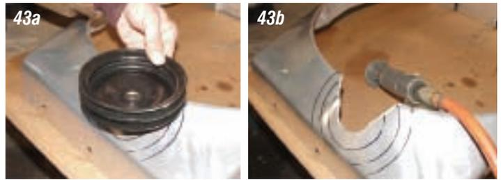
**Photos 43a, 43b & 43c:** Starting slow, trim the shroud with a cut-off wheel or tin snips until the pulley will clear the fan shroud with the pump adjusted all the way out. This will require the fan shroud to be installed and removed several times.
