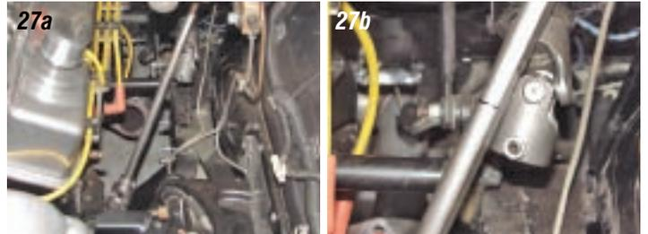
**Photos 27a & 27b:** Install the lower U-joint and shaft on to the rack and pinion unit making sure the set screw is seated in the coped out area on the input shaft. Lay the 3/4" double-D shaft next to the upper U-joint and mark the shaft where it will need to be cut to properly engage the yoke on the joint. The intermediate shaft is long enough to reach the firewall even if a late model tilt column were installed
