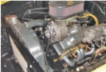
**Photo 58:** Our project car had the alternator mounted to the outboard side of the driver's valve cover. This will no longer work with the pump mounted down low on the driver's side of the
