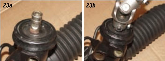
**Photos 23a & 23b:** The input shaft on the rack and pinion unit has a coped-out area for the set screw. With the set screw seated in the coped out area, the input shaft will be flush with the inside U-joint yoke.
