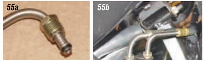
**Photos 55a & 55b:** Before screwing the hose fittings into the rack and pinion, make sure you lubricate the O-rings with a light coat of power steering fluid. When routing the hoses, make sure they are well away from the hot exhaust and the harmonic balancer. We routed our hoses under the side engine mount.
