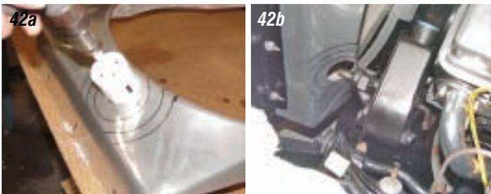
**Photos 42a & 42b:** First, drill a 1-3/4" hole at the center of the markings to line up with the power steering pump shaft when the pump is adjusted as far out as it will go.
