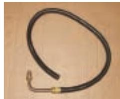
**Photo 53:** The return hose uses a hose clamp at the power steering pump and has a 16 millimeter male O-ring fitting where it attaches to the rack and pinion.
