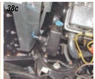
**Photos 38a, 38b & 38c:** The power steering pump P/N 53-28 is held to the bracket with a 3/8" X 3/4" bolt and lock washer in front and a stud at the rear that uses a 3/8" flat washer, lock washer and nut provided with the bracket. With the pump in place, we now see that the shroud will need to be trimmed for the power steering pump pulley. This would be true with a big block or small block engine.
