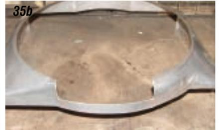
**Photos 35a & 35b:** Future plans include adding air conditioning, so we will install a double groove pulley along with the third track pulley on the balancer. All three pulleys together measure 1-3/4" deep. Using the marks on the fan shroud as the reference point, cut a 1-3/4" deep notch in the shroud. A fine tooth hack saw or tin snips works great to cut the aluminum shroud.
