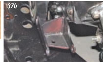
**Photos 37a & 37b:** The pump bracket P/N 53-27 (small block short water pump) is held to the front of the engine with two 3/8" X 3/4" bolt and lock washers provided.
