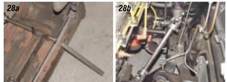
**Photos 28a & 28b:** The shaft can be cut with a hack saw, band saw or chop saw. With the intermediate shaft cut, remove the upper U-joint from the steering shaft, install the now shortened intermediate shaft and lower U-joint to the rack and pinion, install the upper U-joint the intermediate shaft and slide the steering shaft into the upper U-joint.
