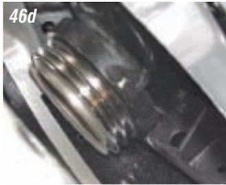
**Photos 46a, 46b, 46c & 46d:** The first groove on our balancer pulleys closest to the harmonic balancer will drive the water pump and alternator. The second groove is for the water pump and air conditioning compressor and the third groove runs the power
