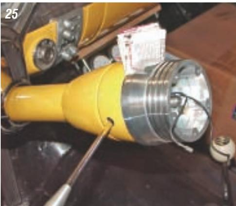
**Photo 25:** Install the steering wheel or steering wheel adapter on the shaft and slide the shaft down into the steering column. Place a piece of cardboard or folded-over paper between the upper mast jacket and steering wheel or adapter. You want to achieve a 1/16" or so gap between the steering wheel hub and steering column.
