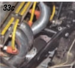
**Photos 33a, 33b & 33c:** The upper bearing in the steering column P/N 53-21 was bad so this was the perfect time to change it before we installed the steering shaft, the steering wheel adapter and the intermediate with U-joints. With everything set and the screws on the U-
