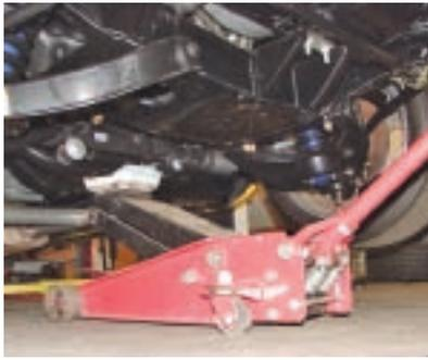
**Photo 14:** The Eckler's Classic Chevy Rack and Pinion crossmember is so strong you can use it to jack up the front end! Other rack kits on the market use a flimsy lightweight support or braces that do not tie the frame rails together.
