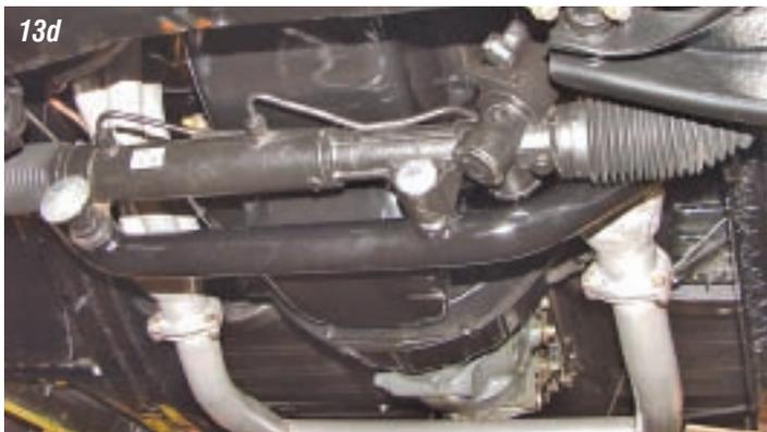
**Photos 13a, 13b, 13c & 13d:** The passenger side of the rack and pinion also has an ear, but this one has a large hole that uses a steel sleeve and two rubber bushings supplied with the kit. A cupped washer is installed on the front side of the ear and a 1/2" flat washer on the back side.
