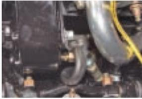
**Photo 56:** The return hose will need to be cut to length and attached to the power steering pump with the supplied hose clamp. The pressure hose screws onto the new brass fitting on the back of the pump.
