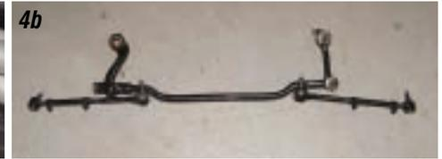
**Photos 4a & 4b:** The idler arm is located on the passenger side of the car and is held to the frame with two carriage bolts, nuts and lock washers. Remove the two nuts and lock washers and the entire steering linkage can be removed from the car.
